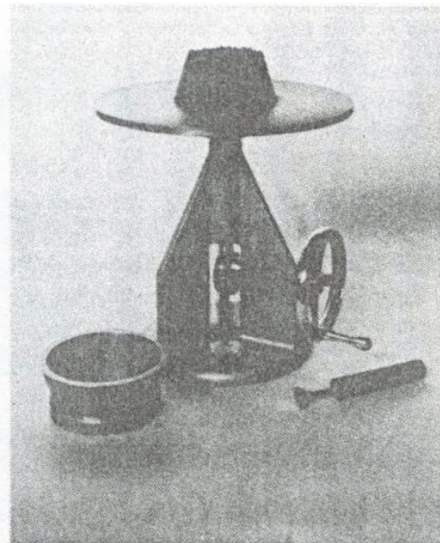
Figure 1.1.2 – Flow table and accessory apparatus
