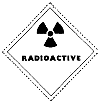
(Minimum length of side: 15 cm) Symbol and inscription black on white ground
